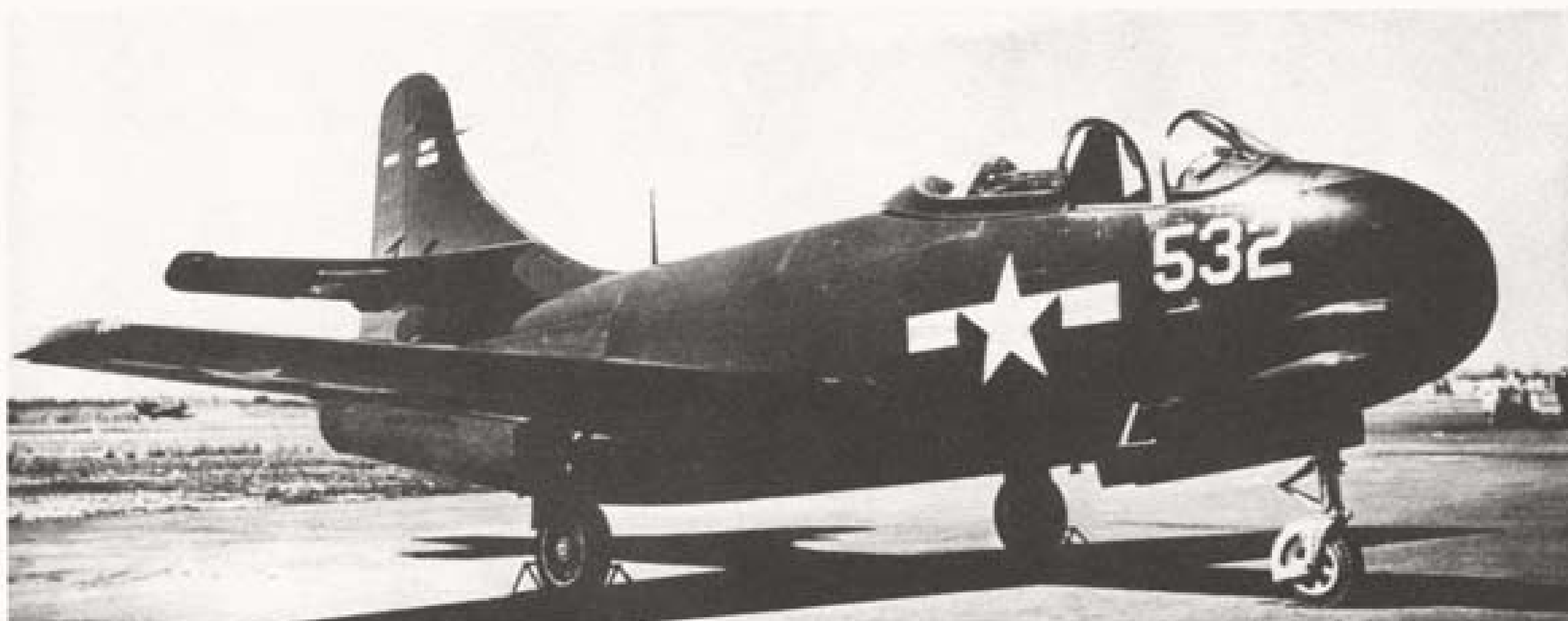
The CHANCE VOUGHT PIRATE XF6U is a carrier based jet fighter with after-burners.
