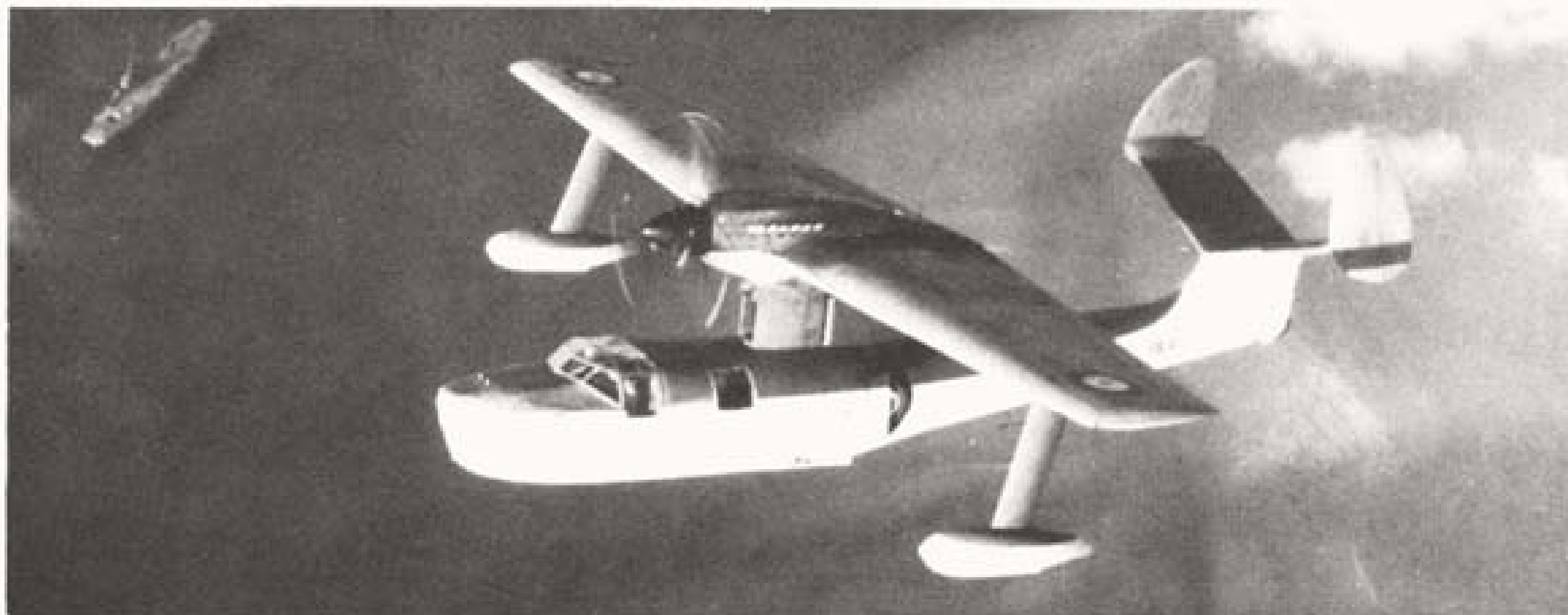
The VICKERS-ARMSTRONGS SEAGULL is a single-engine Naval Amphibian, general utility duties.
