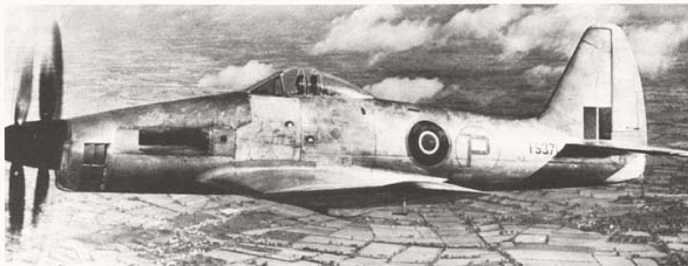
The BLACKBURN WYVERN 1 is a single-seat Naval strike aircraft, the WYVERN 2 will be fitted with a turbo-prop engine.
