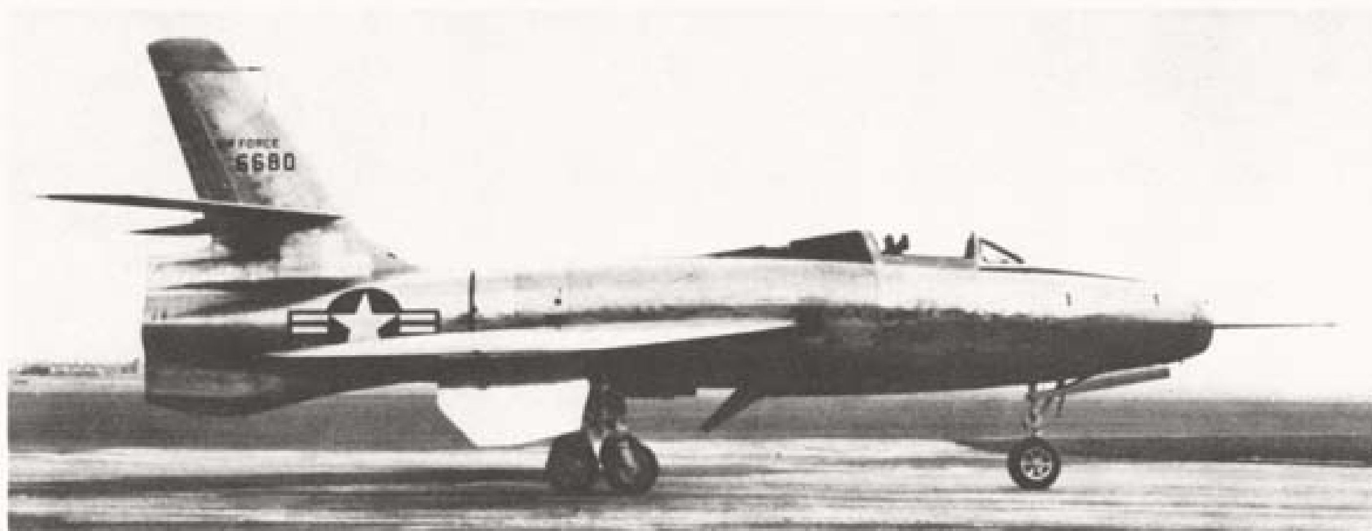
The REPUBLIC XF-91, an experimental model, is a heavy jet-rocket interceptor with reverse tapered wings.
