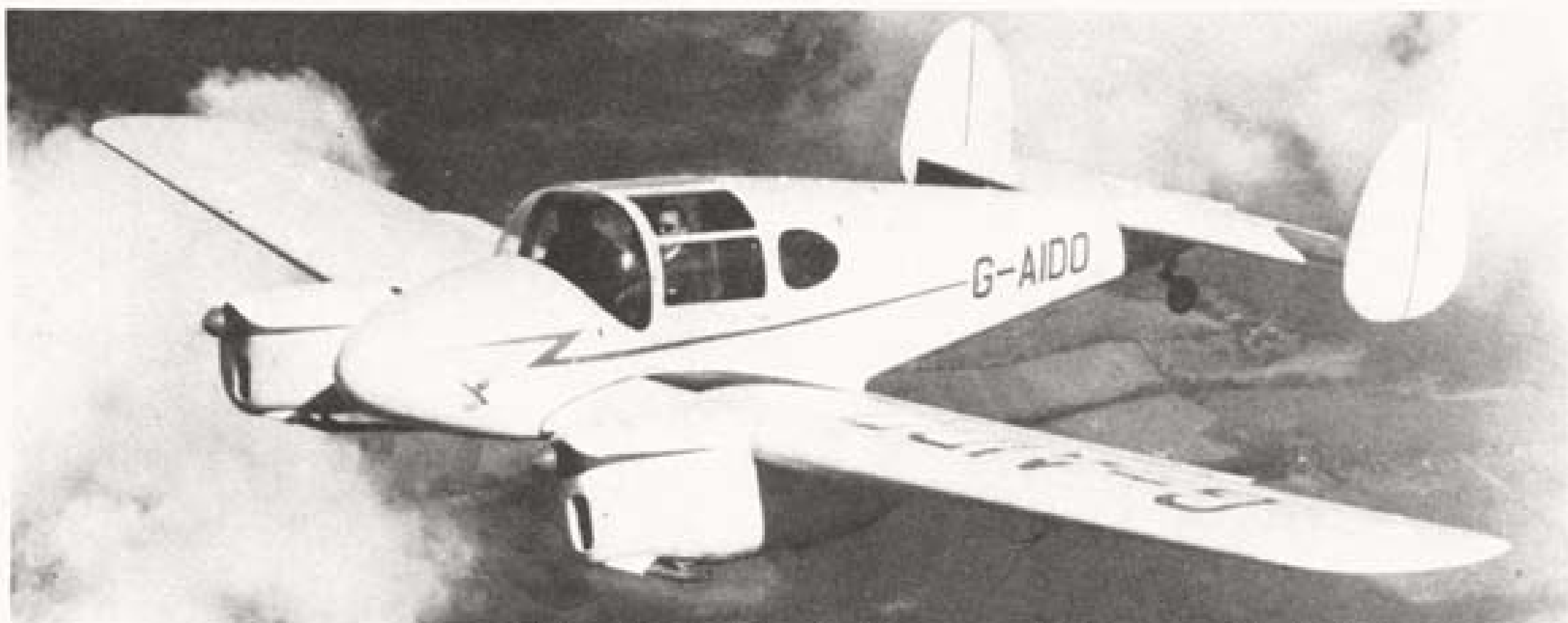
The MILES M.65 GEMINI was developed from the Messenger, carries 3 passengers and pilot.
