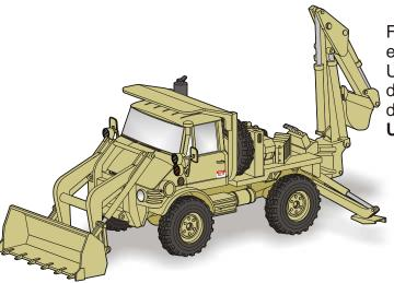
Full resin kit of a truck with dozer blade and spoon excavator. FLU 419 SEE was custom produced for the US Army and US Marine Corps. The truck were combat delpoyed to Kwait and Afghanistan. The kit contains decals and plotter cut foil windows.
