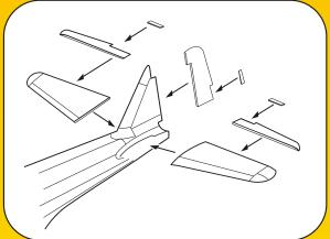
Detailed set with landing flaps and new tail planes for late version of the most famous Japanese naval fighter plane of the Second World War. The tail planes have the control surfaces separated and these can be attached in deflected position. The trim tabs are also separated. Japan/WWII
