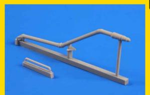
Fixed in-flight refuelling probe used on modernized MiG-29SMPs of the Peruvian Air Force and MiG-29BMs of the Russian and Belarusian Air Forces.
