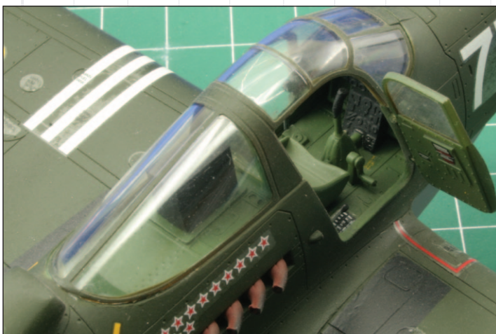
7. Finally, all masking is removed, and the canopy is done.
